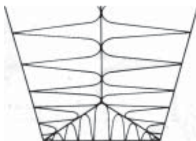
Planes of weakness formed at the junction of columnar columns
